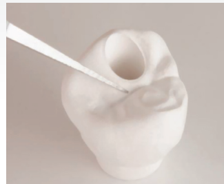
Figure 2: Manual finishing; here, removing the fissures with a square cutter.
