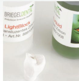
Figure 3 and 4: Opaquing the adhesive surfaces (screw channel) with a light blocker (LightBlock) to conceal the titanium base.
