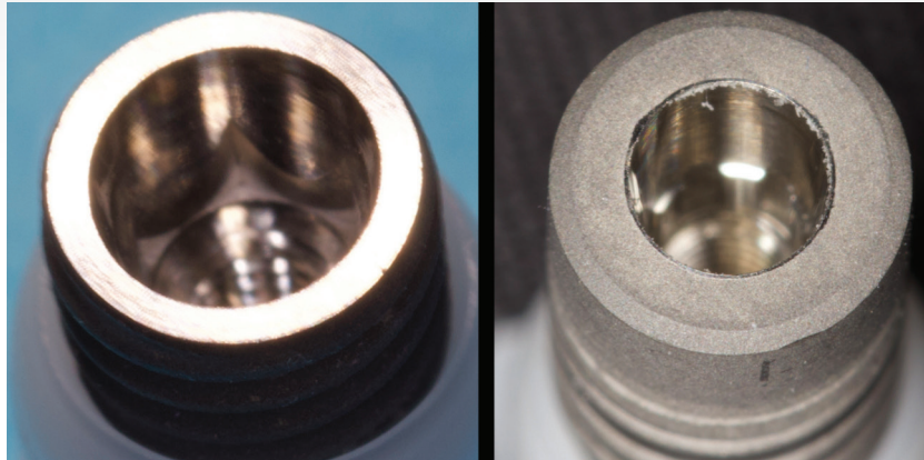
Figure 1: On the left the implant shows a shiny machined platform, compared to the grit-blasted and acid etched surface on the right which has a matt appearance.
