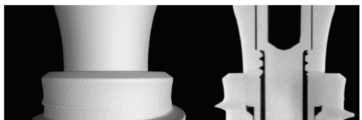
Figure 1: A 3D CT image on the left showing a cone-in-cone connection with the horizontal off-set of platform switching and on the right a cross section of the same implant. The abutment will always be of a smaller diameter in such a connection.
