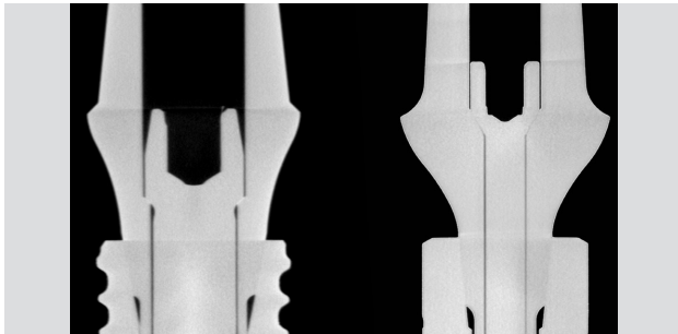
Figure 5: Comparison of two regular platform implant systems, with the implant on the left showing a wider abutment diameter, with slightly less platform switching than the implant on the right, which has a smaller diameter abutment. One could argue that the wider abutment diameter will be stronger and more suitable where occlusal forces are expected to be higher but that would be anecdotal without controlled studies.
