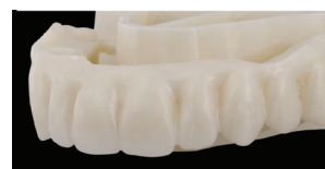
The IPS e.max ZirCAD Prime bridge after sintering.
