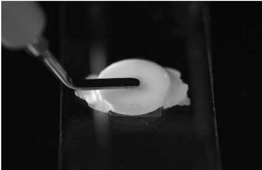
Figure 2. Ultrasonic tip being applied to a specimen.
