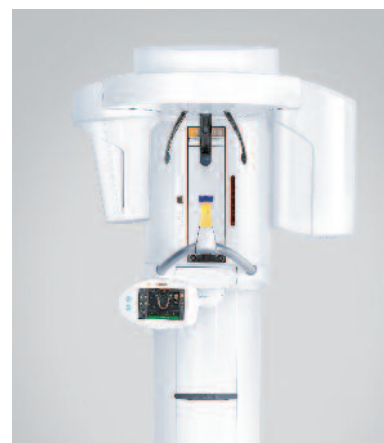
Figure 1: Orthophos SL 3D (Dentsply Sirona) capable of taking limited field of view images with a resolution of 80 µm in the endo mode, ideal for endodontic applications.
